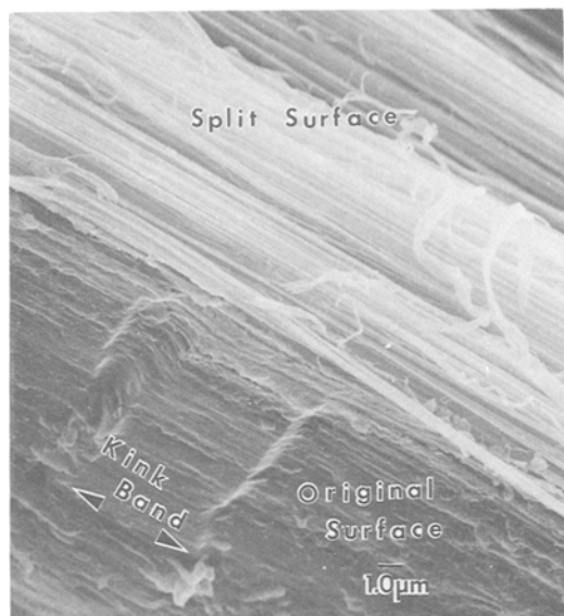
Figure 3 Kink band present on the outer surface but not in the interior of the sample.
